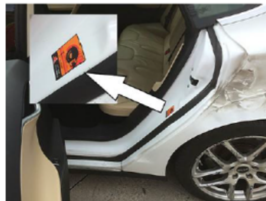
Image of a Factory Identified High Voltage Disconnect
