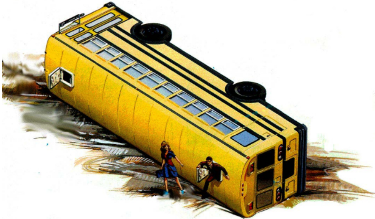
School Bus during Emergency Hatch Operations
